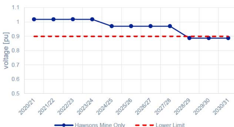
Figure 5.3: Broken Hill 220kV busbar voltage – post contingent
