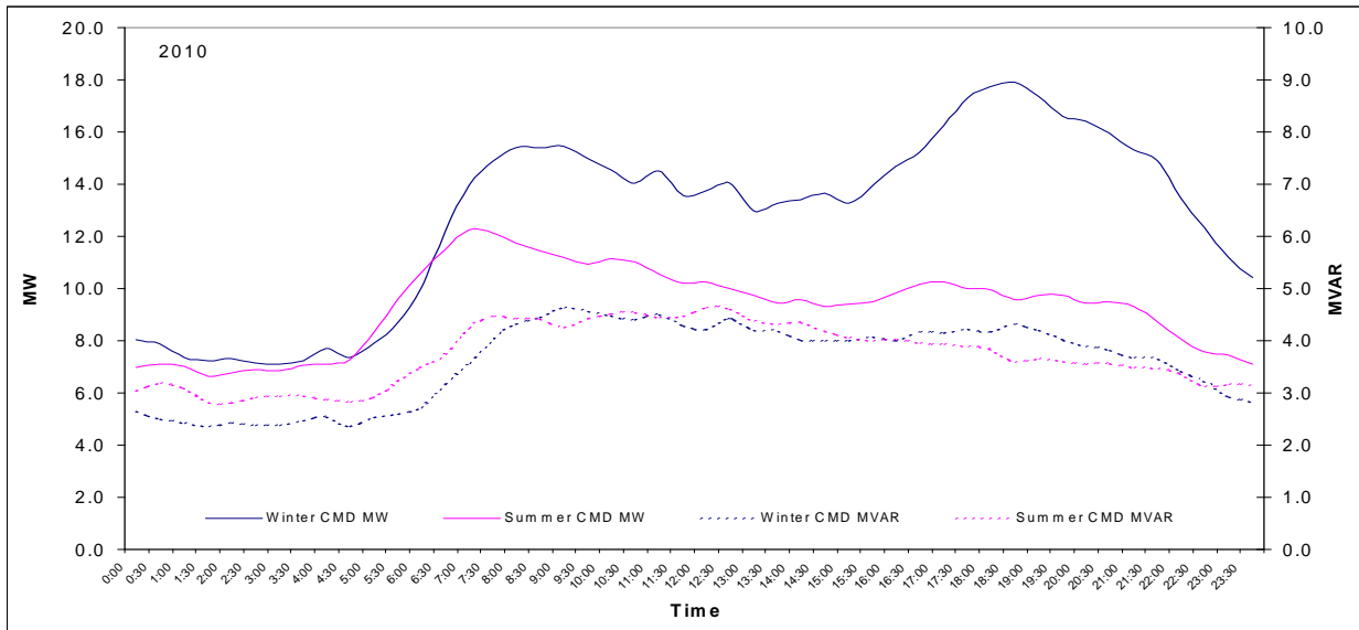
Figure 4-89 Load Profiles: Knights Road Substation Day of Summer/Winter Peak Demand
