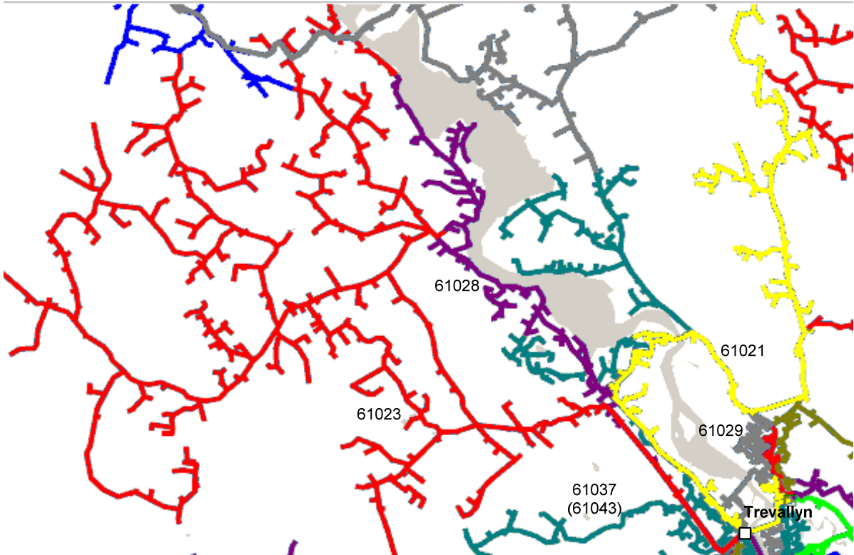
Figure 8-16 Trevallyn 22 kV rural feeders
