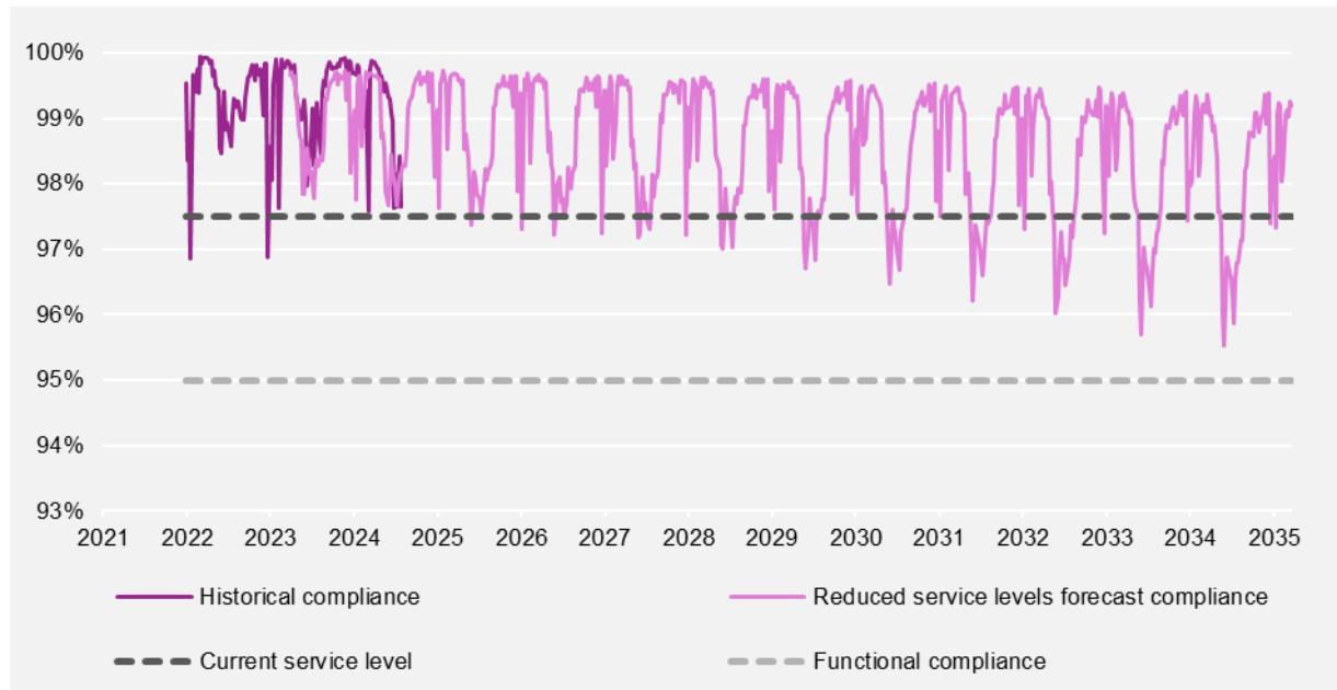
FIGURE 17 FORECAST UNDERVOLTAGE COMPLIANCE UNDER THE BASE CASE (%)
