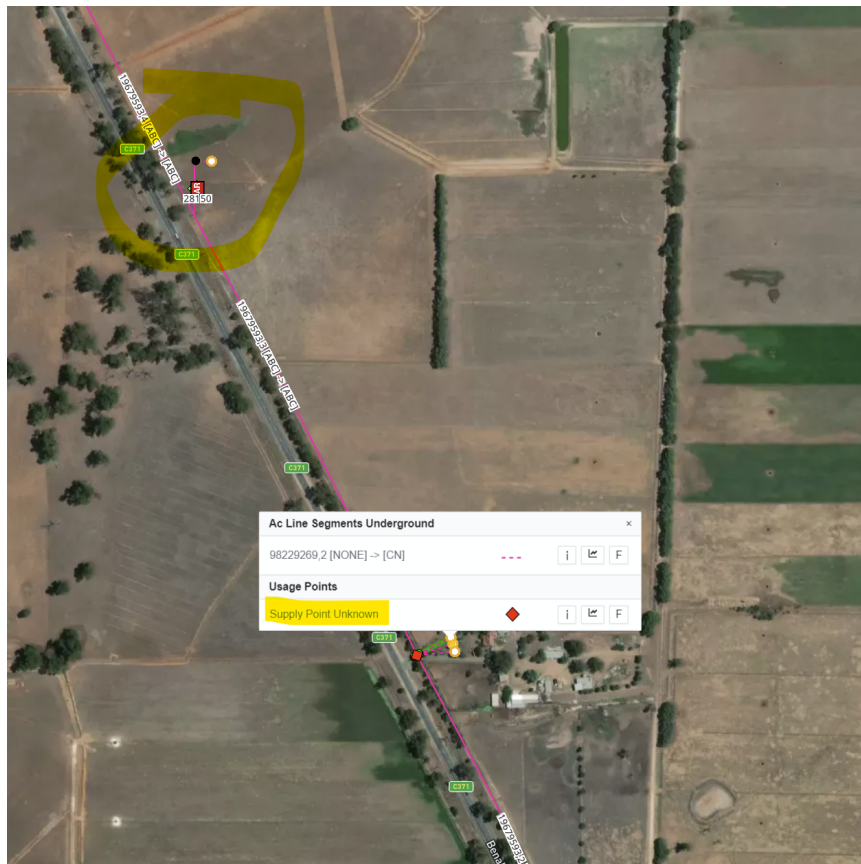
Figure 13 – Incorrect mapping of a solar farm to a domestic transformer
