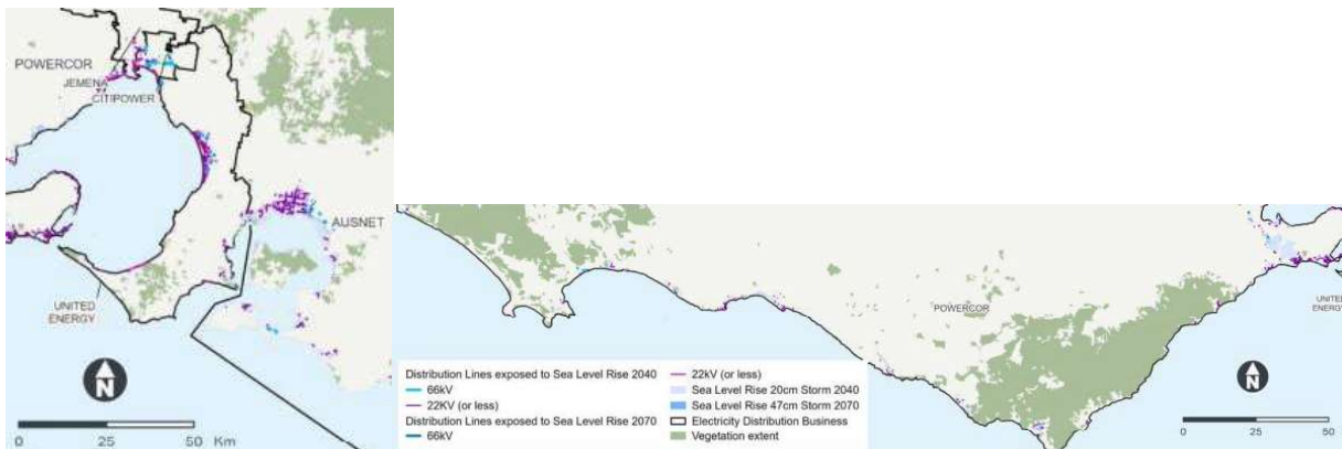
Figure 13: Distribution Lines Exposed to Sea Level Rise
