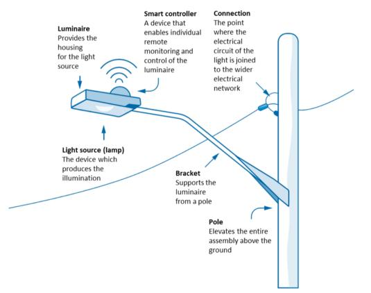
Public lighting systems include all infrastructure associated with providing lighting in public spaces, including the point of connection to the electricity distribution network.
