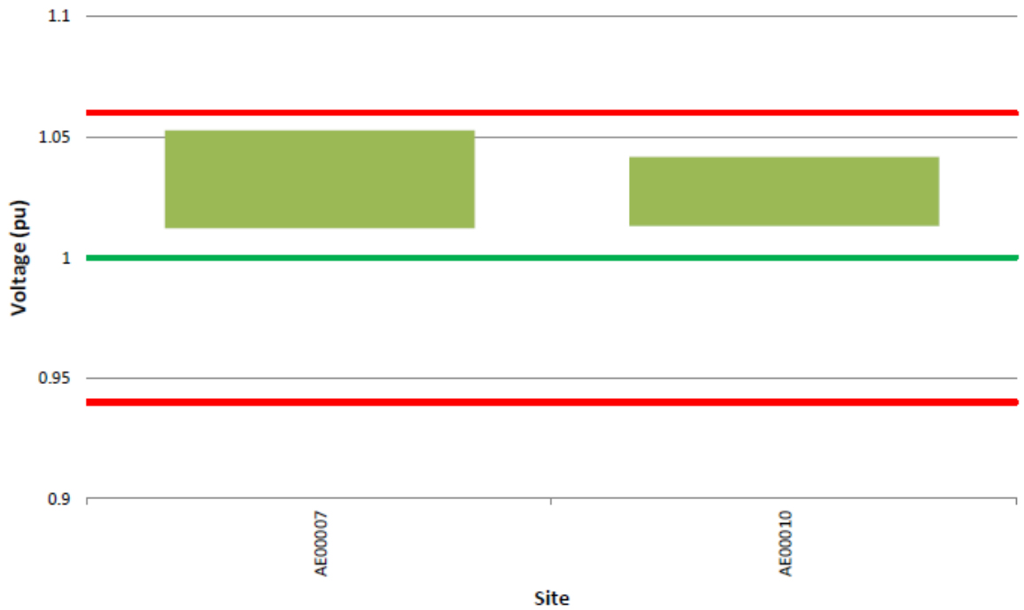
Figure 3-5: Steady-state voltage performance – 6.6 kV sites
