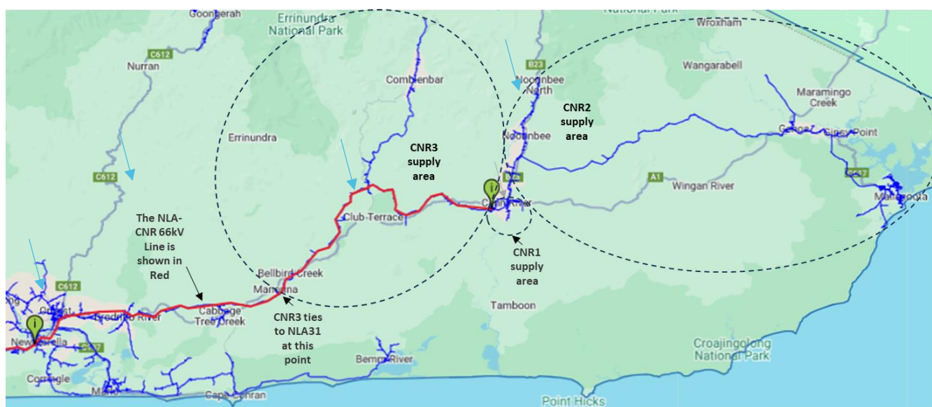
Legend: -Red lines indicate 66kV -Blue lines indicate 22kV -Green pins indicate zone substations -Dashed lines indicate highlight the supply areas for CNR feeders
