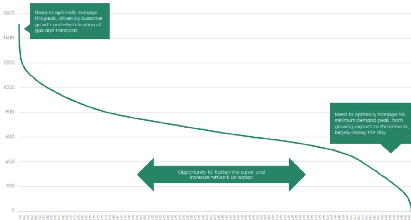
Figure 9: Demand duration curve and need to manage both ends of the spectrum (illustrative)
