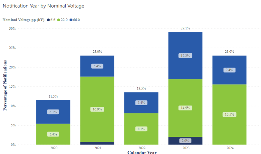
Figure 6 Zk notifications during the period 2020 - 2024 by service voltage
