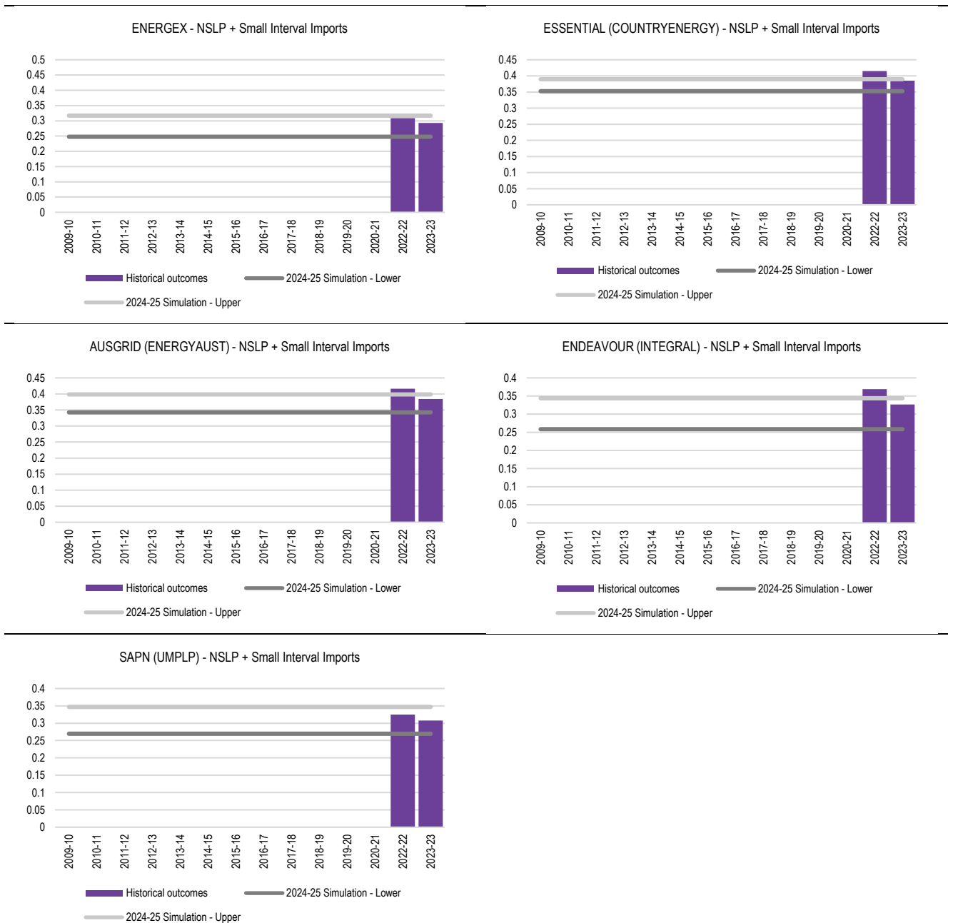
Figure 4.14 Comparison of load factor of 2024-25 simulated hourly demand sets with historical outcomes – NSLP and small interval meter demand
