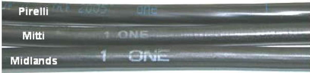
Figure 1: XLPE Service Cable photograph showing identification markings
