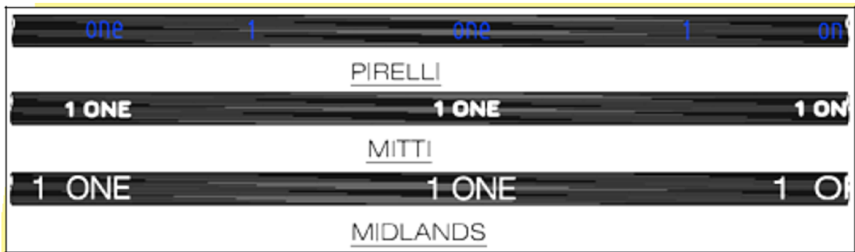
Figure 2: XLPE Service Cable drawing showing identification markings
