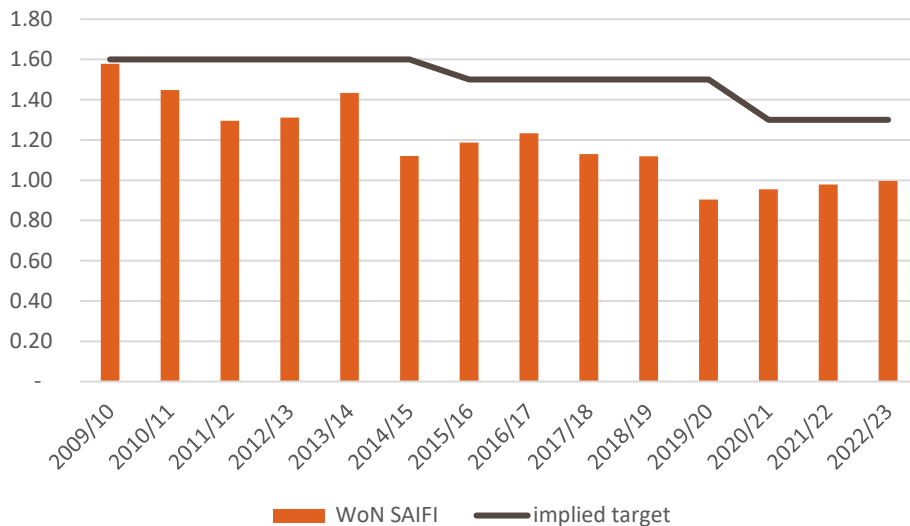
Figure A.7: Distribution system unplanned system average interruption frequency index normalised (USAIFI) and implied whole of network jurisdictional target.
