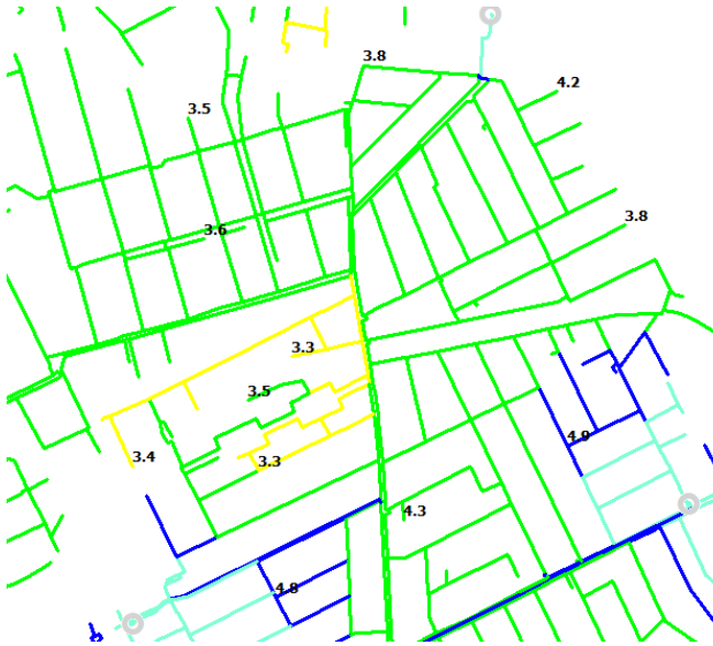
Figure 42: Campsie network modelling in 2026 prior to reinforcement
