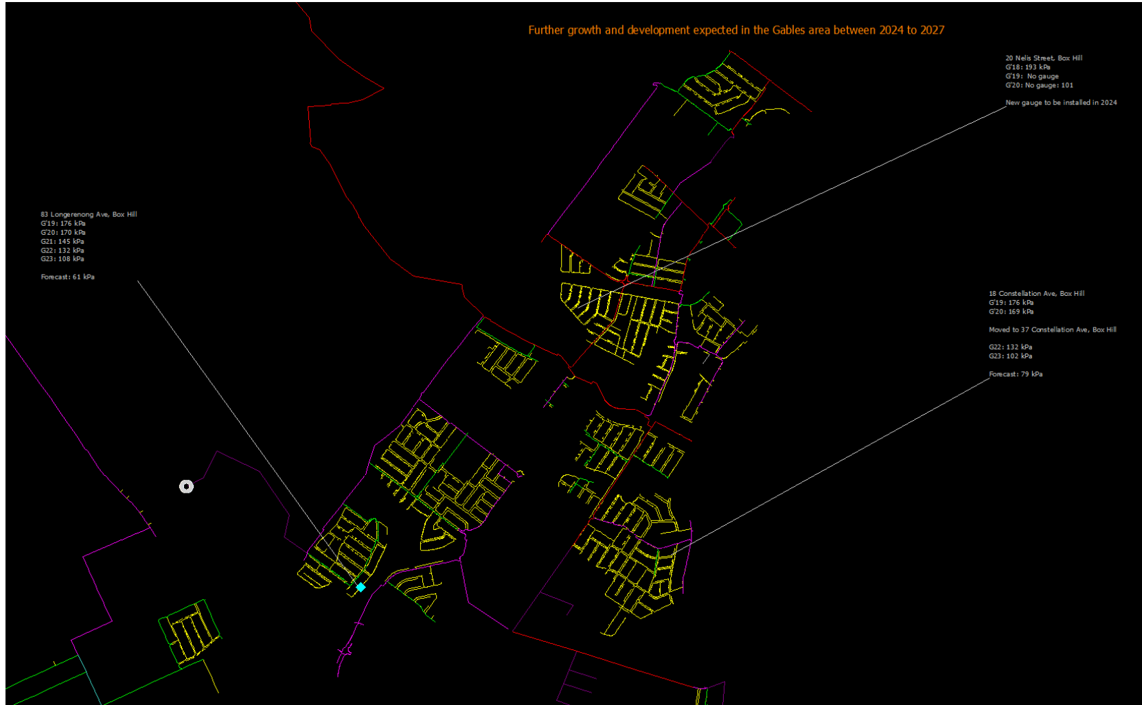
Figure 4: Synergi model forecast before after implementation of CDP increasing pressures at the end of the network (61 kPa)
