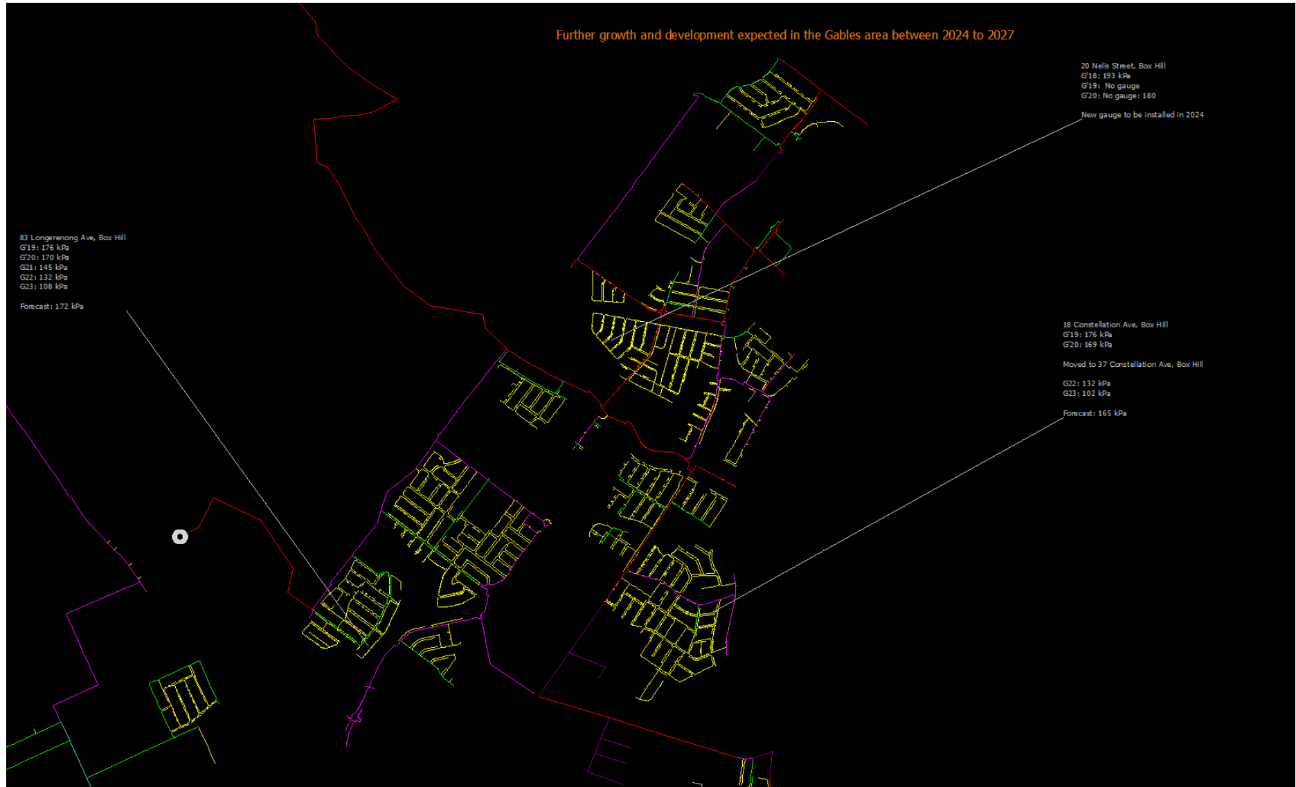
Figure 5: Synergi model forecast after implementation of CDP increasing pressures at the end of the network (165 kPa)
