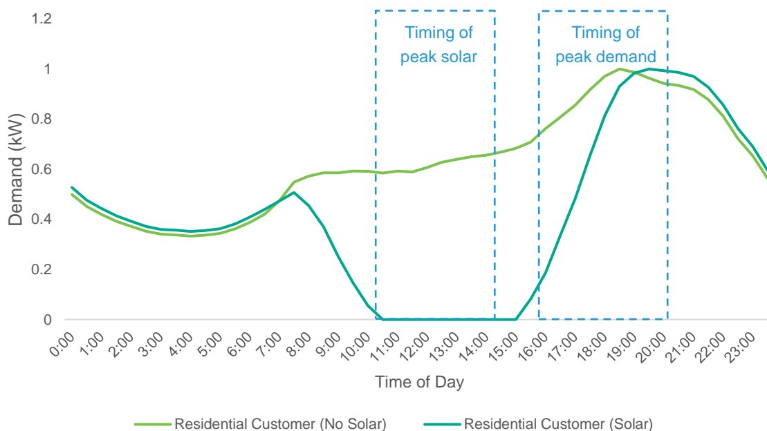
Figure 12: Generation from solar PV does not coincide with system peak demand
