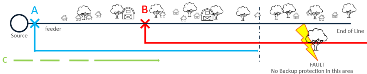
Figure 4: Adequate vs Inadequate Backup Protection
