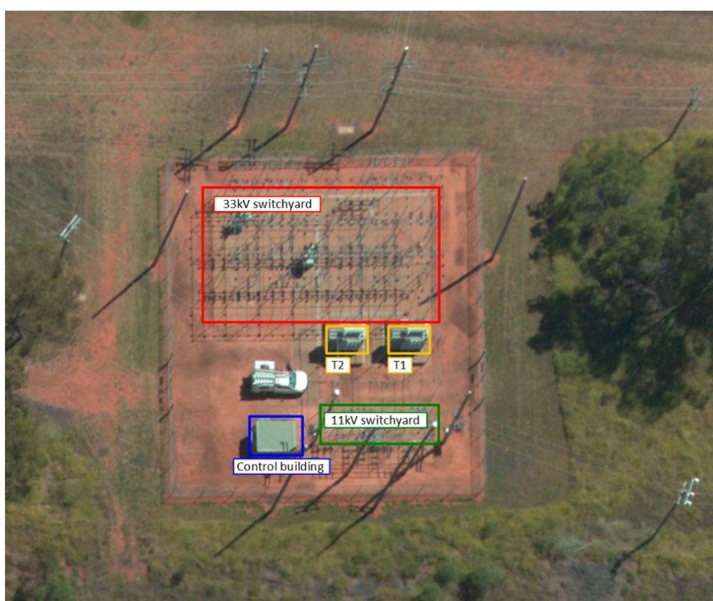
Figure 3 – CHTW site general arrangement
