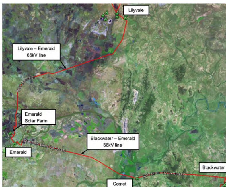
Figure 1: Existing network arrangement (geographic view)
