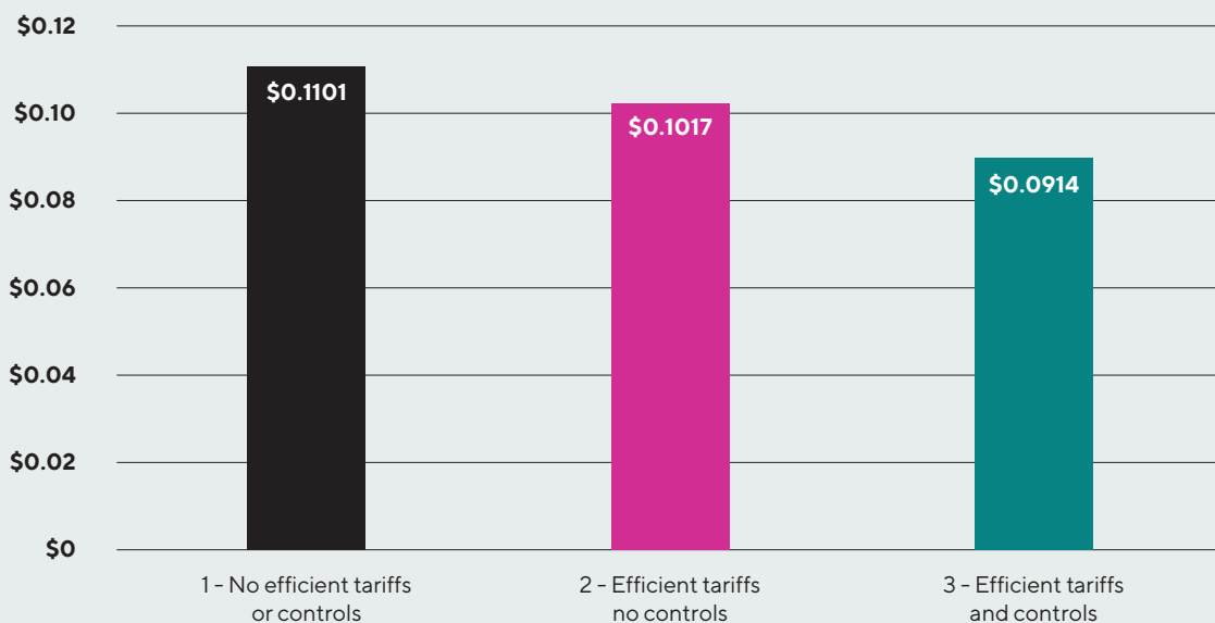
Figure 3 – Cents per kilowatt hour by 2050 for Ergon customer base under each scenario (real 2024)
