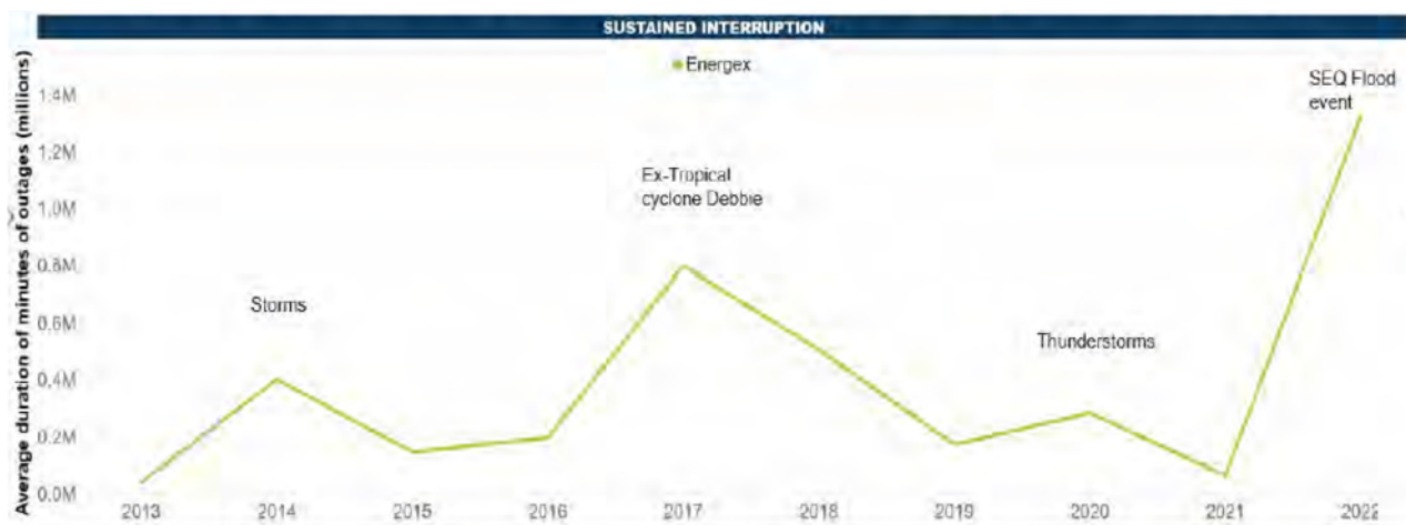
Figure 12 – Average duration of minutes of outages, including major event day and other exclusions in Energex’ networks (2013-2022)
