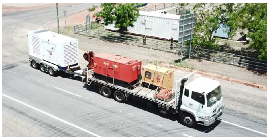
Figure 1 – Deployment of LV mobile generator
