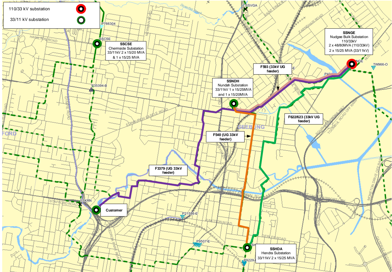
Figure 2 – Existing network arrangement (geographic view)
