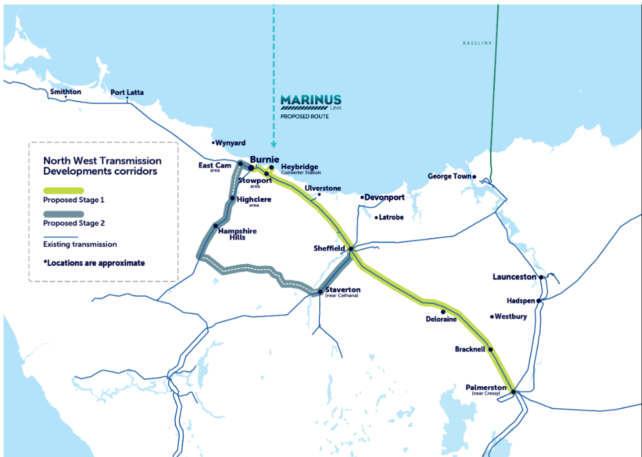
Figure 9-1 North West Transmission Developments revised scope
