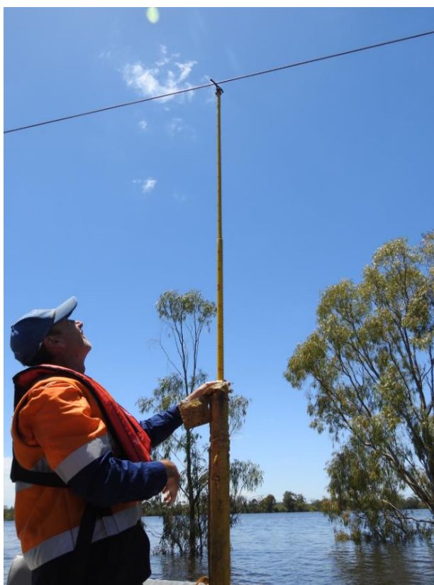
Figure 7 - Measuring clearance of conductors to surface of flood waters.
