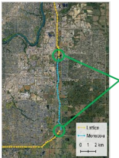
FIGURE 2: MONOPOLES USED IN 10KM OF TRANSMISSION LINE TO GAIN COMMUNITY SUPPORT
