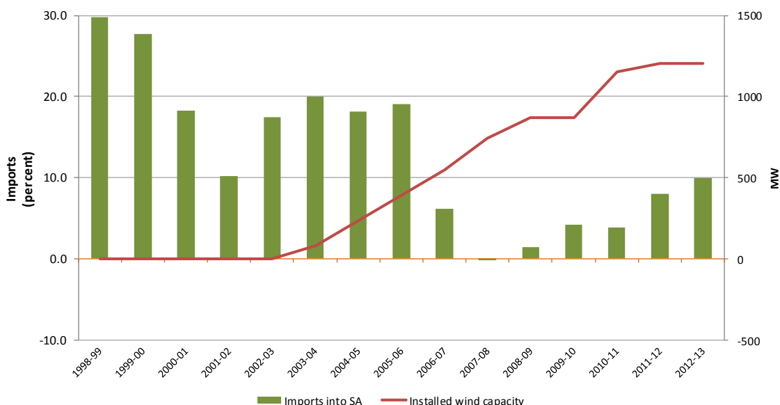
Figure 5: Interregional trade as a percentage of South Australian energy demand compared with installed wind capacity
