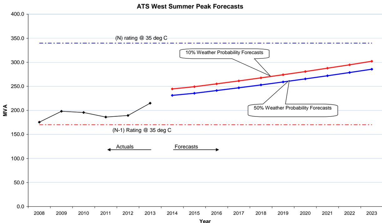
The “N” rating on the chart indicates the maximum load that can be supplied from ATS West with all transformers in service. The “N-1” rating on the chart is the load that can be supplied from ATS West with one 150 MVA transformer out of service.
