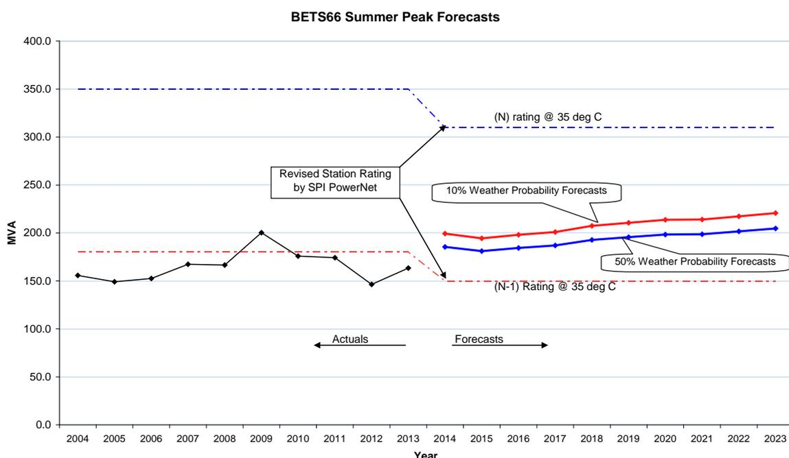
The (N) rating on the chart indicates the maximum load that can be supplied from BETS with all transformers in service. Exceeding this level will initiate automatic load shedding by SPI PowerNet’s automatic load shedding scheme.
