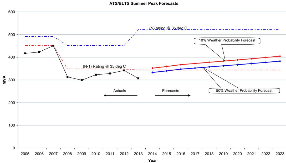
The “N” rating on the chart indicates the maximum load that can be supplied from ATS-BLTS with all transformers in service. The “N-1” rating on the chart is the load that can be supplied from ATS-BLTS with one 150 MVA transformer out of service.
