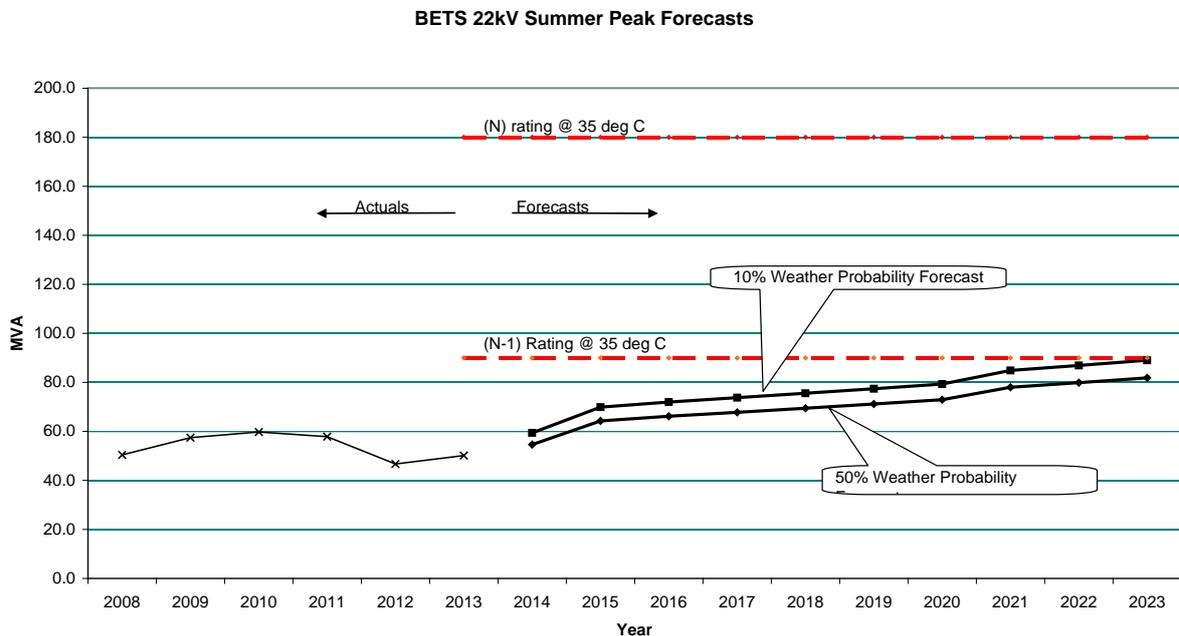
The (N) rating on the chart indicates the maximum load that can be supplied from BETS with all transformers in service. Exceeding this level will initiate automatic load shedding by SPI PowerNet’s automatic load shedding scheme.
