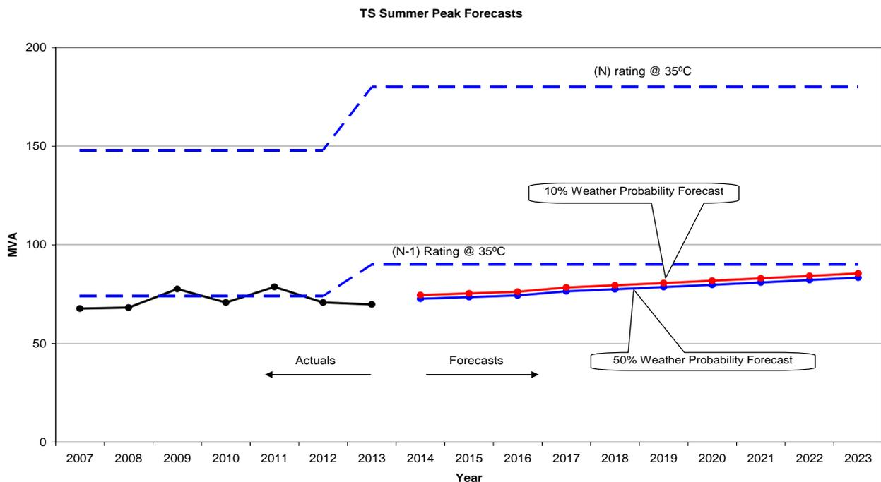
The “N” rating on the chart indicates the maximum load that can be supplied from BLTS 22 kV Terminal Station with all transformers in service. The “N-1” rating on the chart is the load that can be supplied with one 75 MVA transformer out of service.
