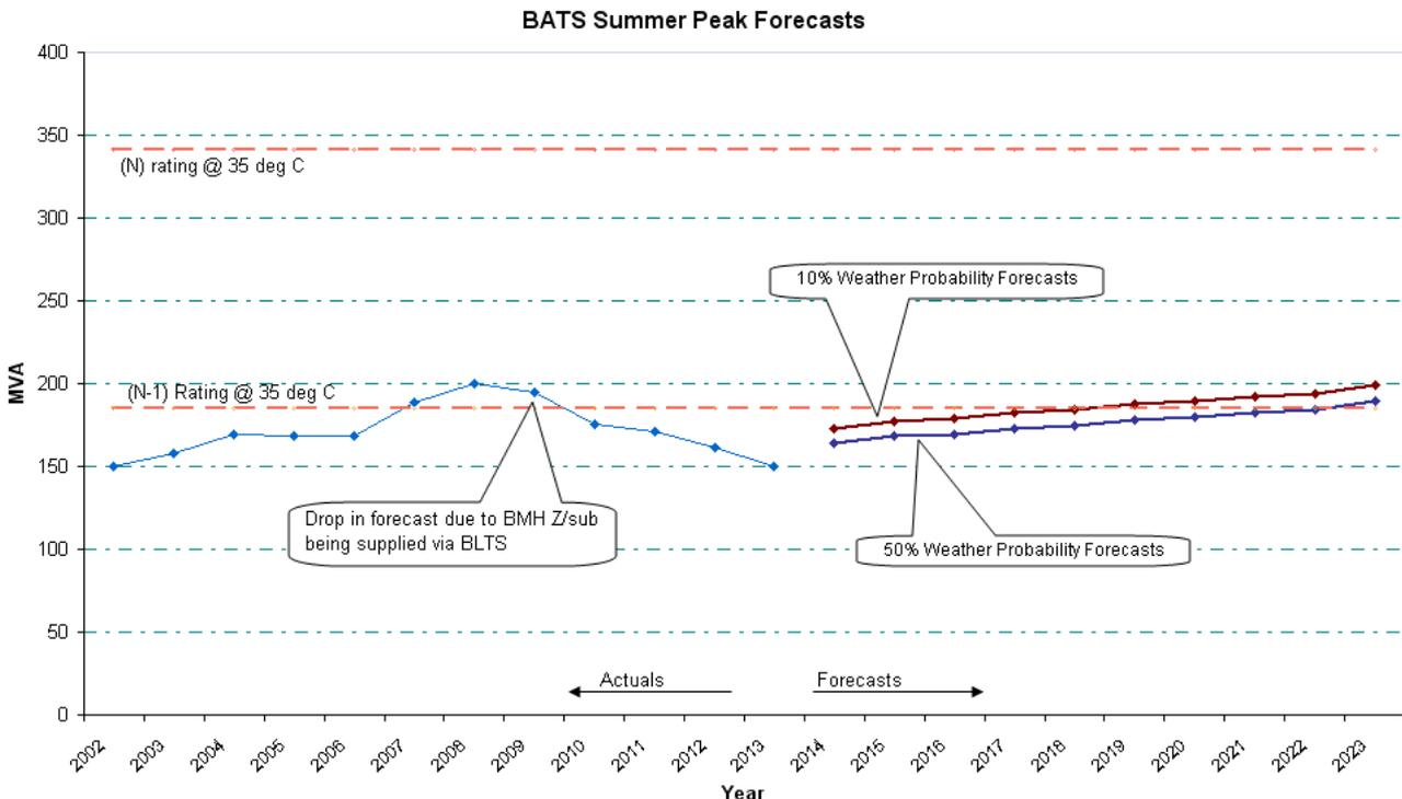
The (N) rating on the chart indicates the maximum load that can be supplied from BATS with all transformers in service.
